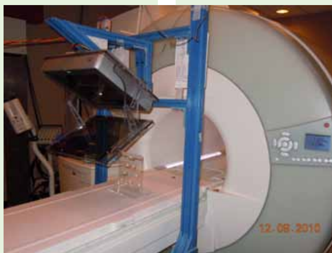
Frame-mounted Image-Overlay system prototype in conjunction with a clinical 1.5 T MR scanner (Magnetom Espree, Siemens Healthcare, Erlangen, Germany).
